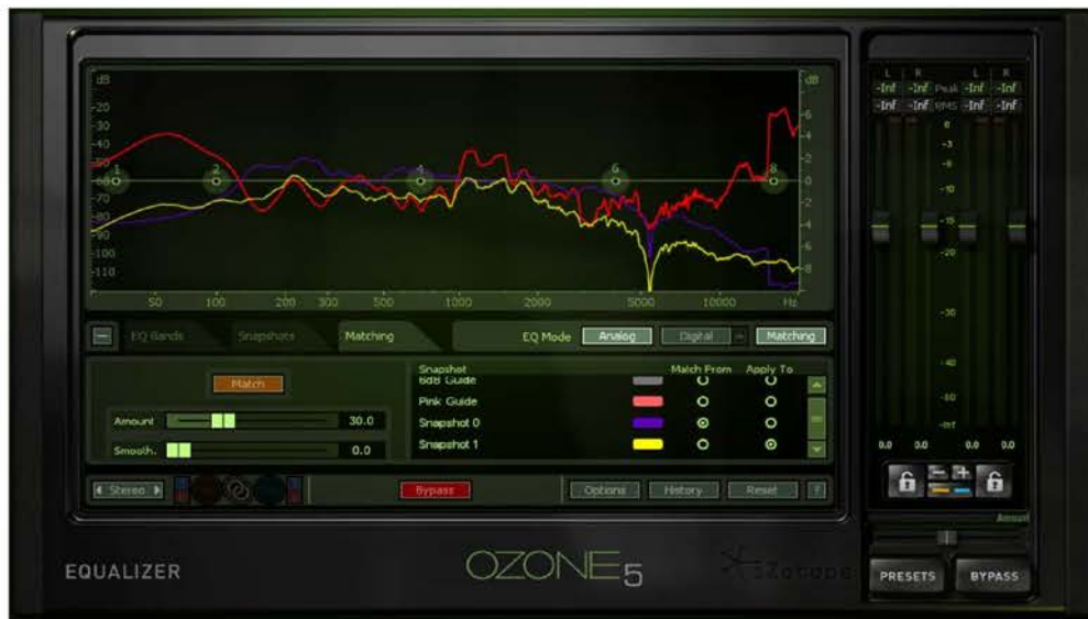
Fig. S1. Matching of frequency spectra. After intensity normalization, we used Ozone 5's frequency matching function to capture frequency distributions of hurdling (yellow curve) and tap-dancing recordings (purple). Using hurdling as a reference, the difference curve (hurdling – tap-dancing, red) was computed to adjust the frequency distribution of tap-dancing to match those of hurdling recordings. The amount of frequency matching (see 'Amount' slider, bottom left) was set to make sure that no clipping would occur after applying the equalization. Note that the smoothing parameter was set to zero, ensuring a close approximation of both distributions.
