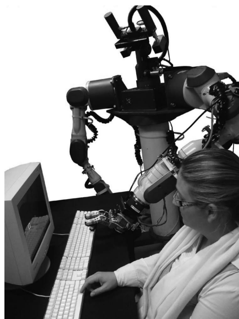
Figure 1. Experimental setup: Social Simon task shared between a human and a humanoid robot.
