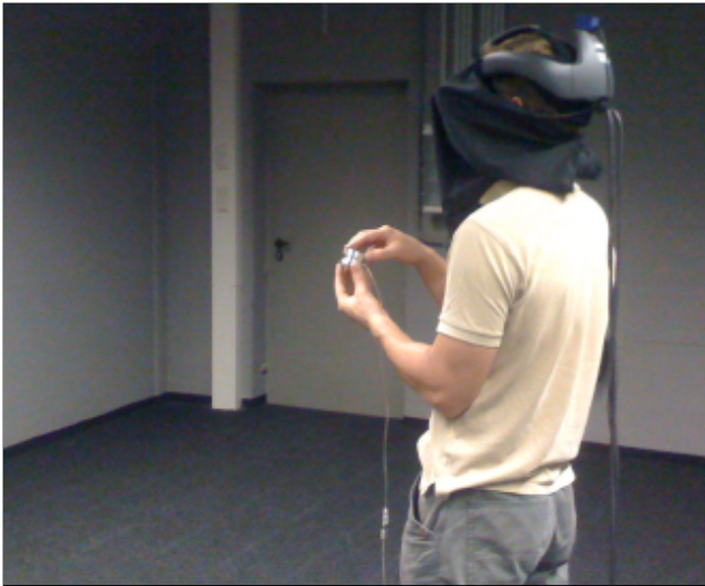
Fig. 5. Photo from the experiment showing a subject with the ProView SR80 HMD adjusting the GFOV with the PowerMate.
