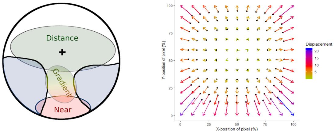
**Figure 1.** Schematic of a progressive additive lens and its distortion vectors in the FOV. The gradient corridor between the distance (green) and near view (red) zones leads to unavoidable side-effects in the periphery e.g. skew on both sides of the lens (blue).
