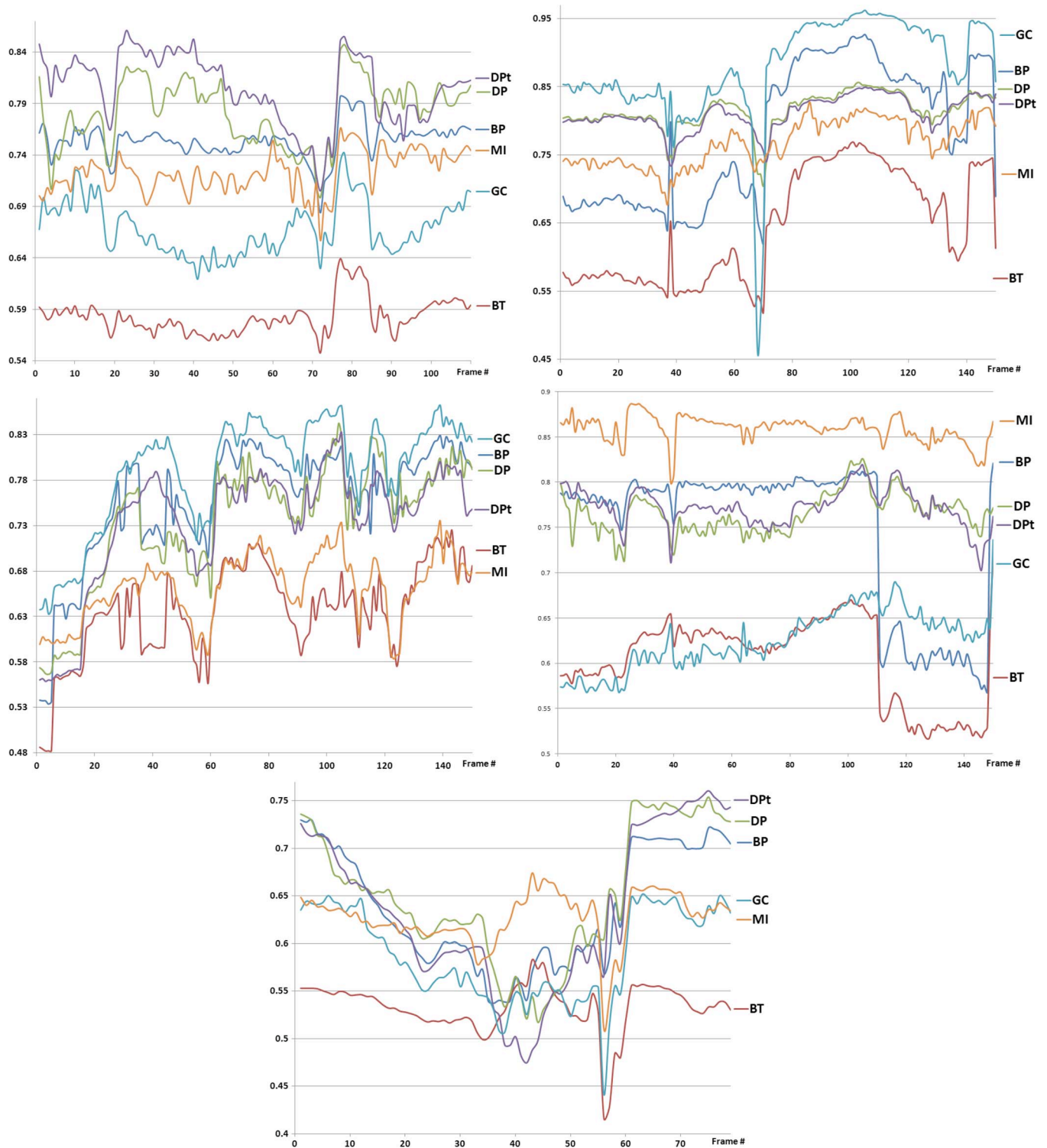
Fig. 3. Performance of stereo algorithms on five different situations using a NCC measure (a larger value is “better”) on trinocular sequences. (Top row) Ordinary Conditions (left) and Illumination Artefacts (right) sequences. (Middle row) Inner City at Night (left) and Brightness Difference (right) sequences. (Bottom) Close Objects sequence.
