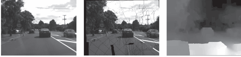
Fig. 4. Application for a sequence in set 5. (Left) Third view. (Middle) Virtual view for the disparity map shown on the right. The matching algorithm applied was BP stereo analysis. The specularity (left), which is apparent both in the recorded left and right images, causes a “defect” in the calculated disparity data.
