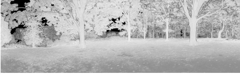
Figure 2. Panoramic projection of 3D data of a range-image, The grey values encode the intensity of the reflected laser beam.
