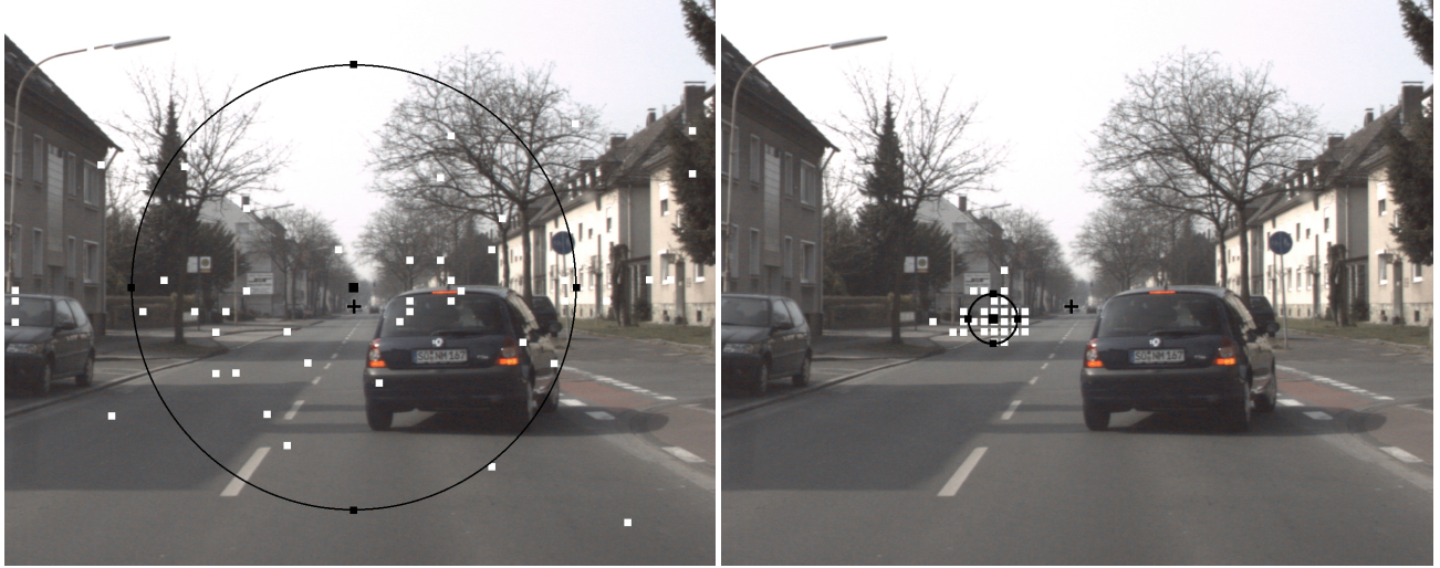
Figure 5: Individual results of heading estimation on flow fields obtained from real camera recorded image sequences. Left: unfiltered flow, right: space-variant filtered flow
