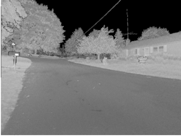
Figure 1: Projection of a range-image onto a plane. The ratios between width and height and the focal length are chosen as 1 and 0.7 respectively.
