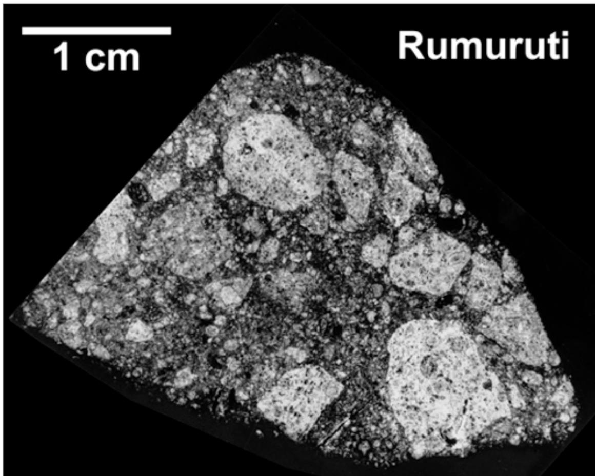
Fig. 6: Overview of the R chondrite regolith breccia Rumuruti. The photographed hand specimen consists of light- and dark-colored fragments embedded in a clastic matrix. The abundance of large clasts is roughly 50%. See Schulze et al. (1994) for details.
