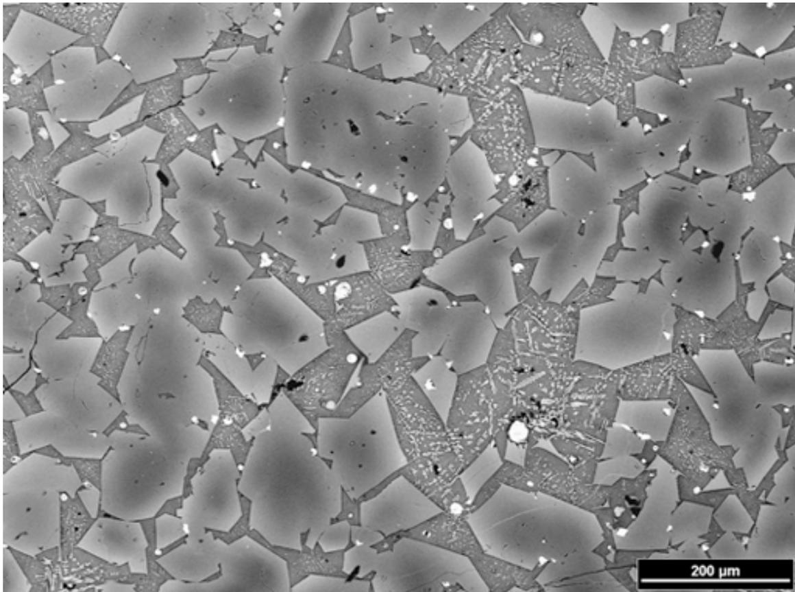
Fig. 7: Typical texture of an impact melt clast within the R-chondrite Dar al Gani 013. Euhedral to subhedral, zoned olivine grains are embedded in a mesostasis containing tiny, skeletal crystals of pyroxene. Light grains are either chromite or Fe-sulfid. Image in backscattered electrons.
