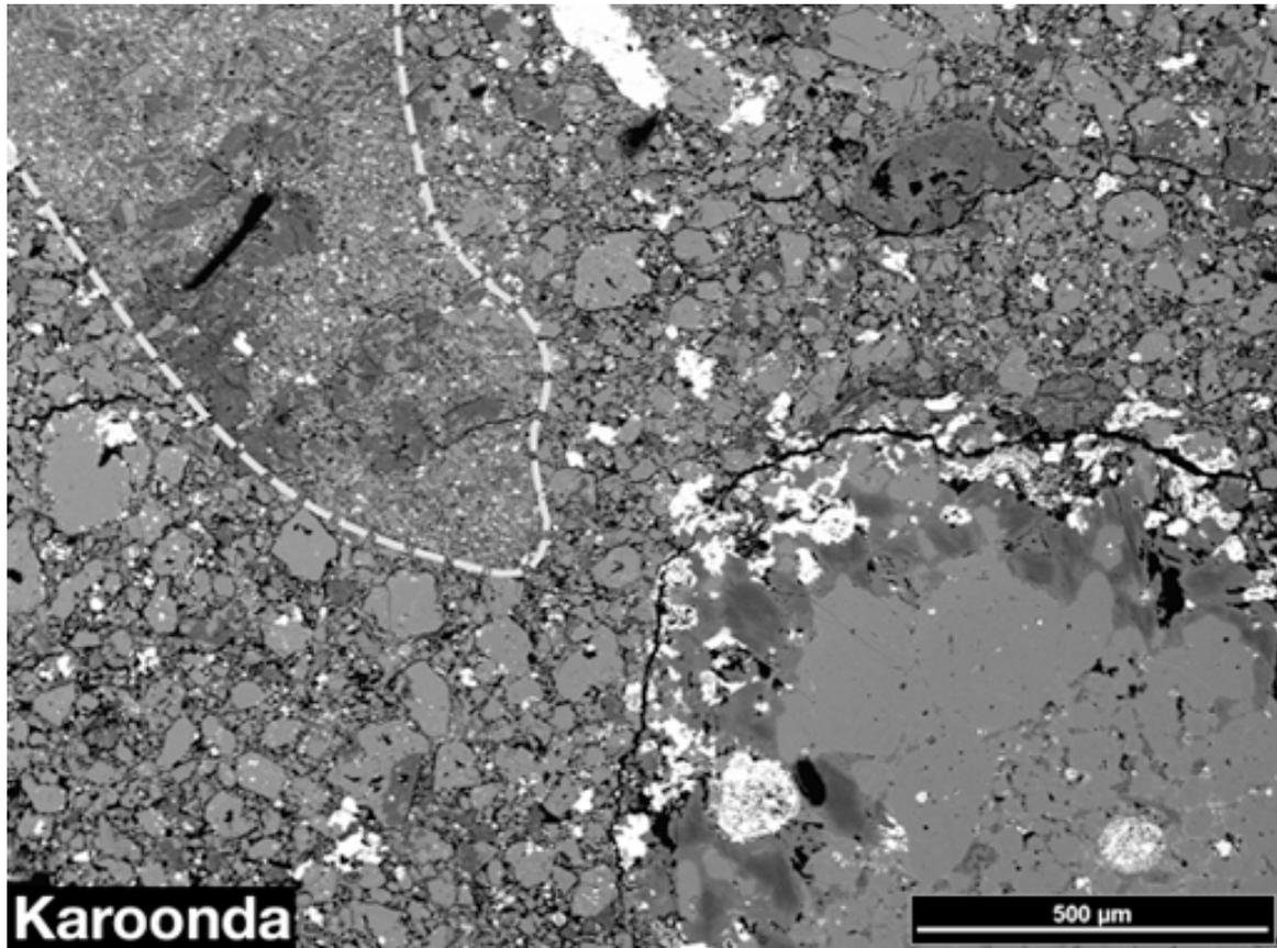
Fig. 10: Brecciated nature of the Karoonda CK chondrite. A fine-grained (upper left) and coarse-grained fragment (lower right) are embedded in a fine-grained clastic matrix. Image in back-scattered electrons.
