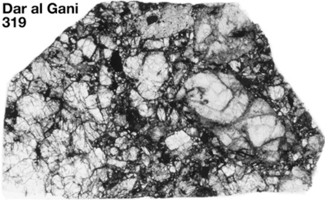
Fig. 13: Overview photograph of the polymict ureilite Dar al Gani 319 showing the fragmented character of the sample (1.4 cm in largest dimension).
