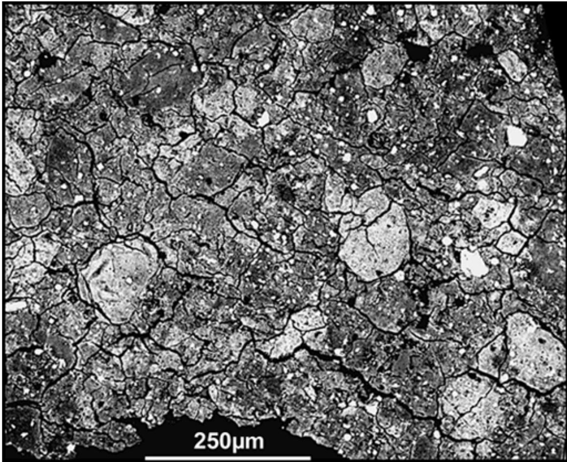
Fig. 8: Part of the severely brecciated CI chondrite Orgueil. Individual fragments are variable in composition as indicated by different grey tones. Image in backscattered electrons; modified after Morlok (2002).
