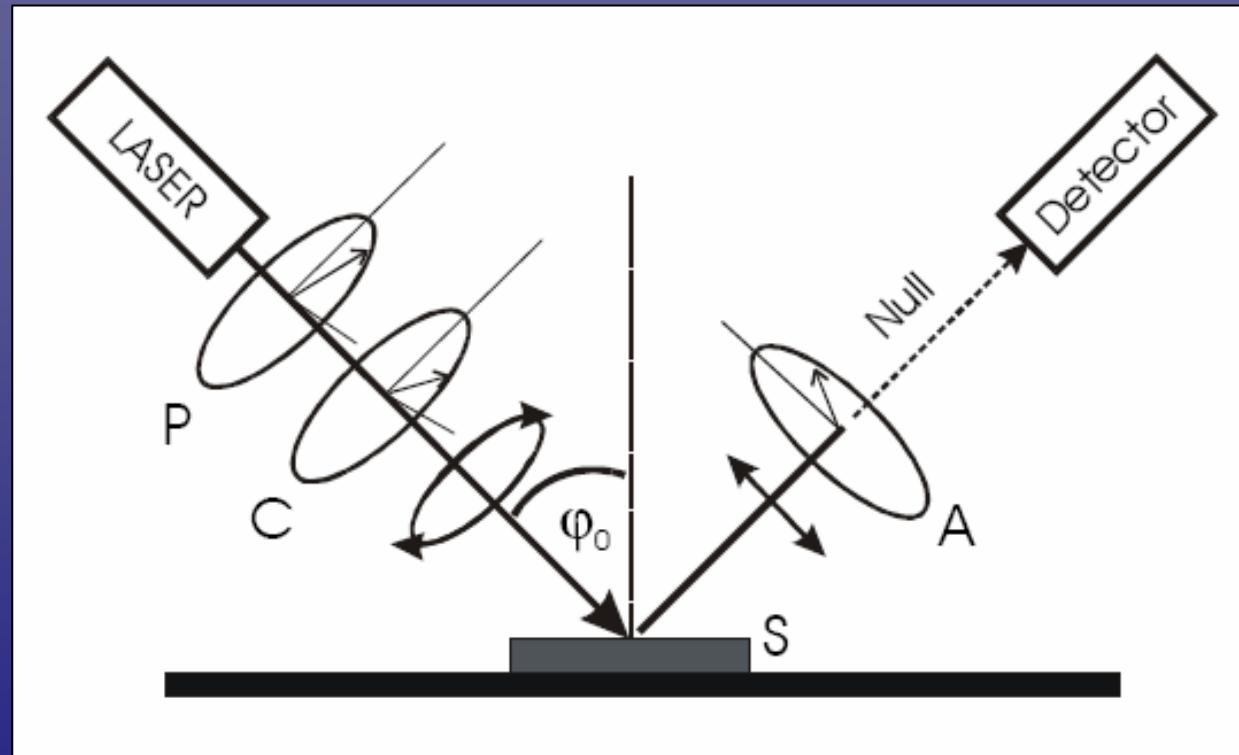
P: Polarisator, C: Compensator, S: Substrat, A: Analysator
