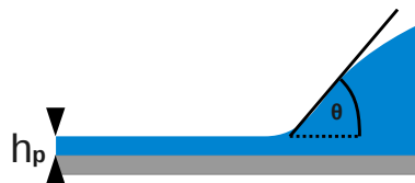
Figure 4.2.: Sketch of a contact line placed on an ultrathin precursor h_p and of the apparent contact angle \theta .
