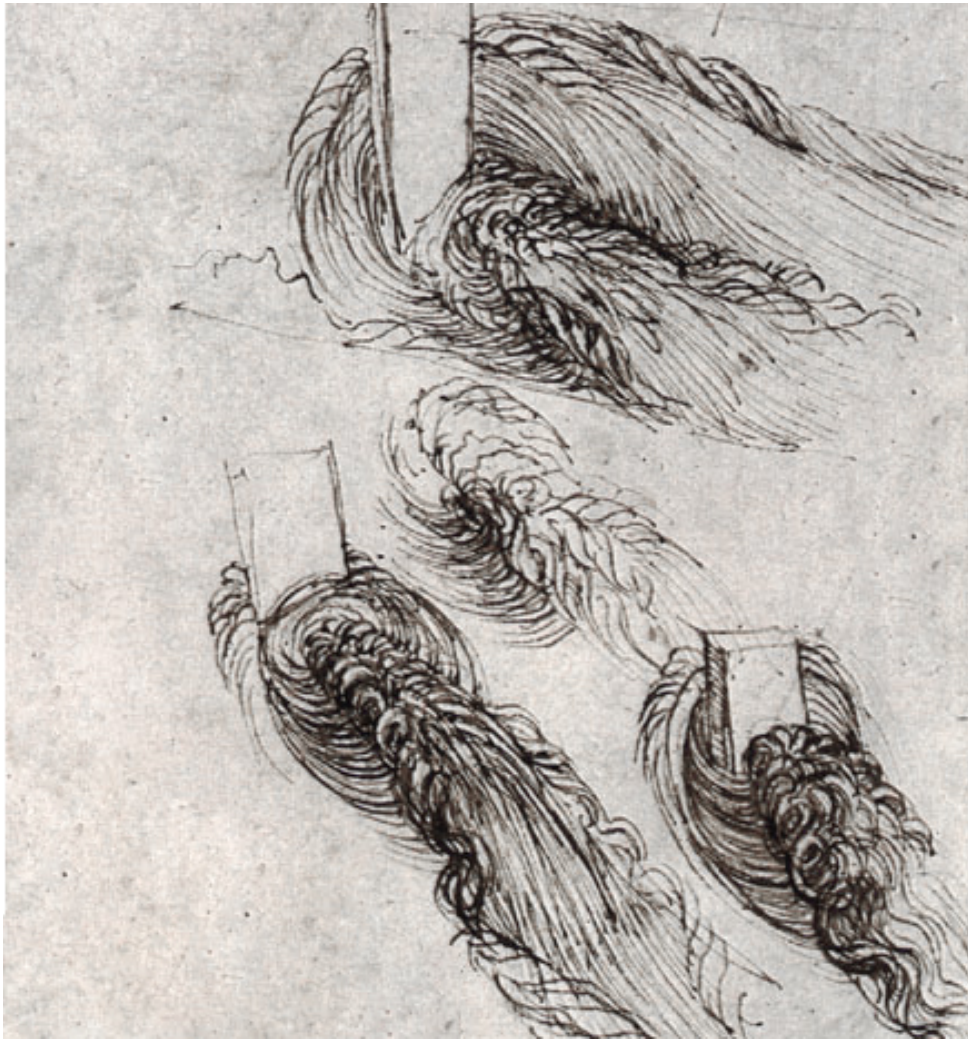
Figure 3.2: Leonardo da Vinci's sketch of water passing a row. A separation of vortices with different length scales and intensities can clearly be observed.
