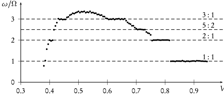
Fig. 5.2: Synchronization plateaus obtained from one-dimensional simulations of transfer onto a prepatterned substrate with L_p = 400 and \rho = 6 \cdot 10^{-3} .
