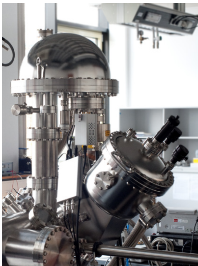
UHV set-up for photoelectron spectroscopy at the CeNTech.
