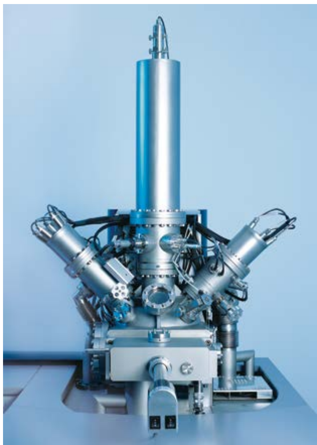
ToF-SIMS equipment for chemical surface analyses
