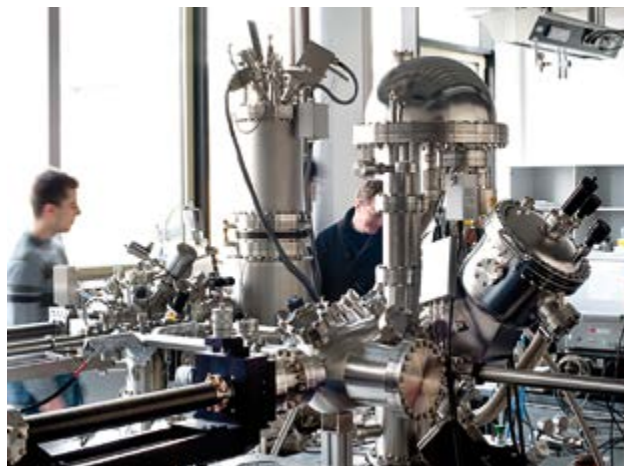
To achieve highly defined experimental conditions, the experiments are carried out under ultrahigh vacuum conditions and at temperatures close to absolute zero.
