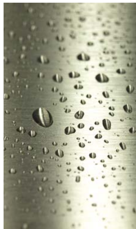
Metallic surface made hydrophobic through nanocoating
