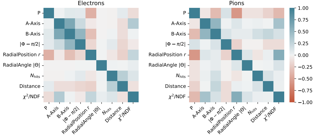
Figure 6.3: Correlations matrices for the input data in the classification methods, for electrons and pions separately. Blue values belong to a positive correlation negative to a red correlation.
