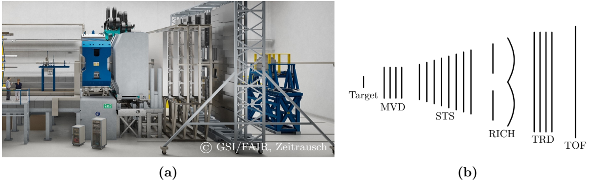
Figure 2.2: The layout of the CBM experiment in the cave [9] (a) and as a schematic drawing (b). Different subdetectors are lined up behind the target which is placed inside a superconducting dipole magnet.
