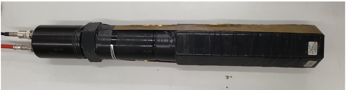
Figure A.2: The detector with the BaF 2 scintillator.
