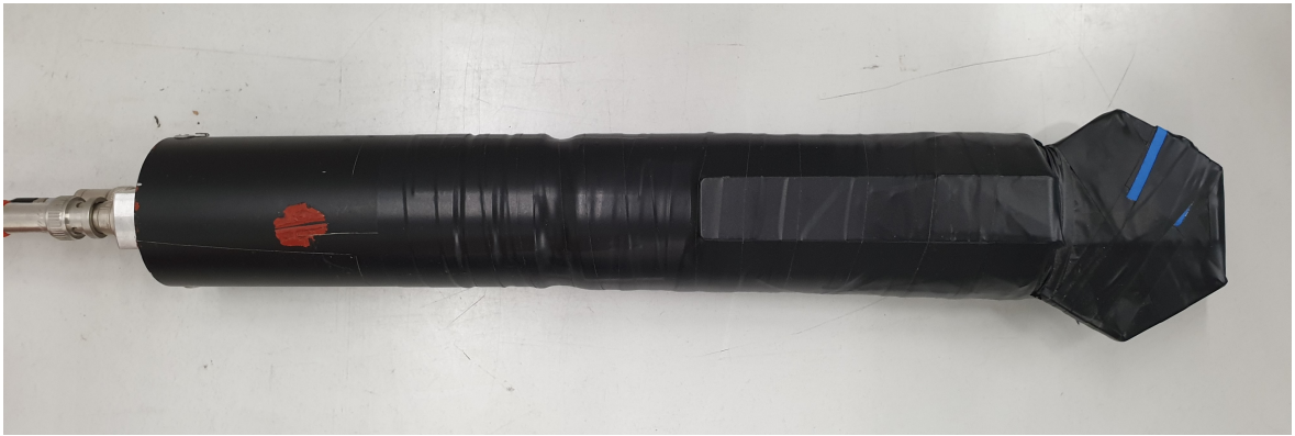
Figure A.1: The detector with the plastic scintillator.
