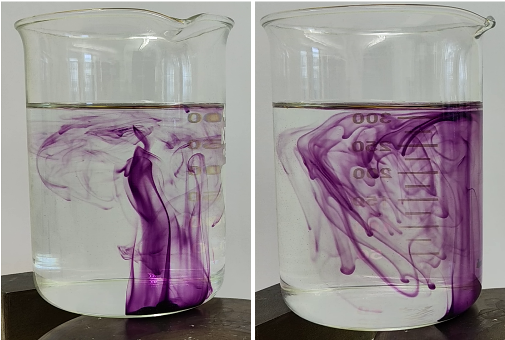
Figure 46: A beaker with tap water is partly placed on a heat source. Food dye indicating a convective current of warm water rising above the heat source (left) and a circular flow is seen from the side (right).
