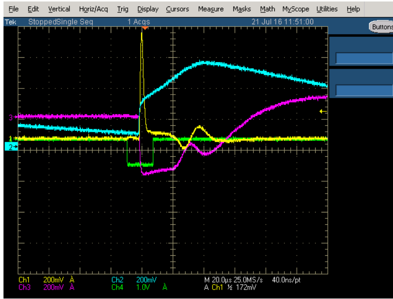
Figure 4.6: Measured pad signal of an event after the preamplifier (purple), after the mainamplifier (yellow) and the corresponding anode signal (blue). The green curve show the gate triggered by the scintillator.
