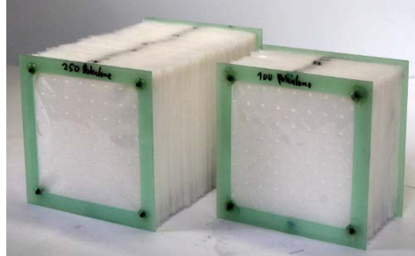
Fig. 6.17: Self-Supporting Micro-Structured Foil Radiator K is presented on the left and Kshort on the right side. The combination of both prototypes is called K++.
