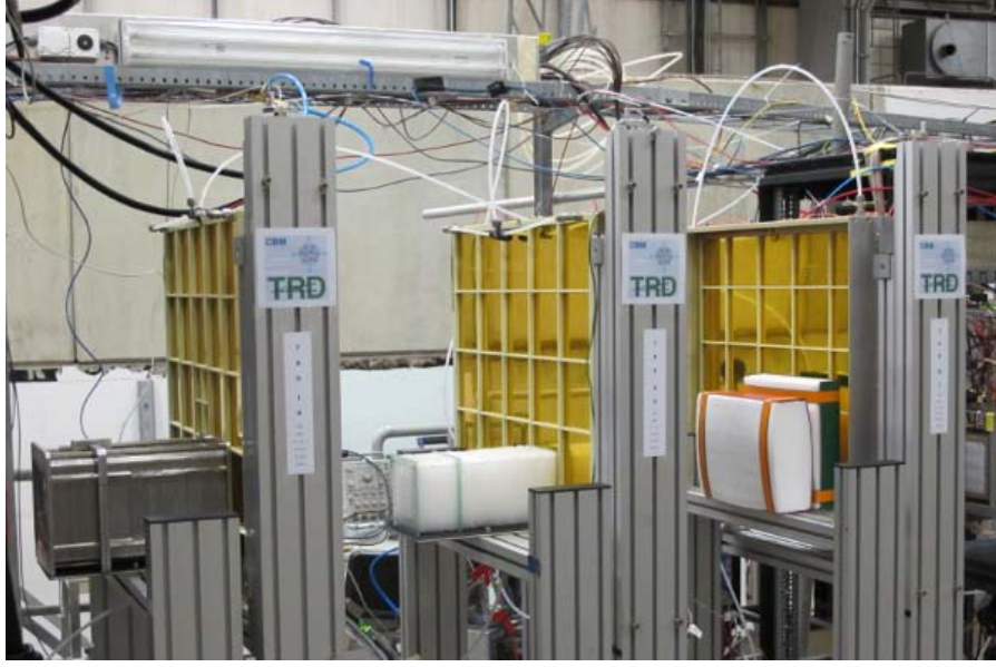
Fig. 8.21: Münster prototypes R I, N II and J III in the beam line T9 at CERN, with radiator prototypes B++, K++ and G30 from left to right side.
