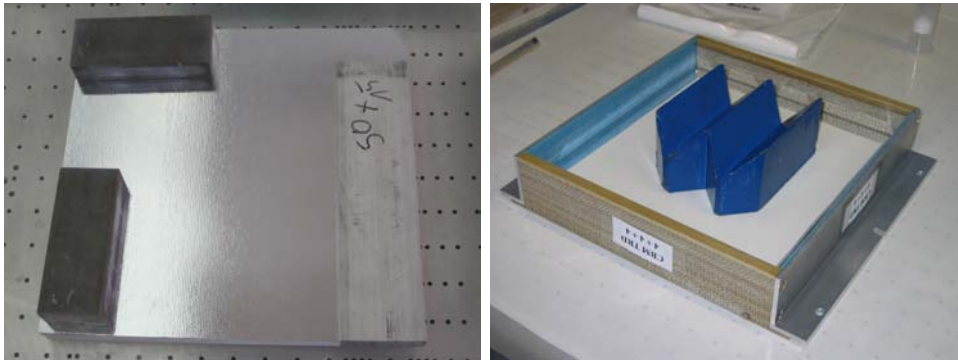
Fig. 5.21: The front-panel built from two Rohacell/carbon-fiber/Mylar plates (8 mm thickness) is glued together (left) and afterwards applied to the chamber body made from four Wacosit profile parts (right).
