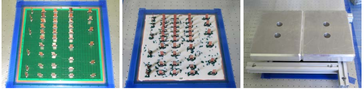
Fig. 5.23: Gluing of the back-panel to the pad-plane.
