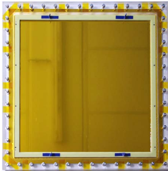
Fig. 5.31: Kapton foil window for the open TRD geometry is shown, after stretching in the oven.
