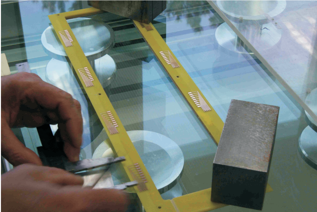
Fig. B.6: Anode plane before gluing on the central kapton-alu plane [MP09]
