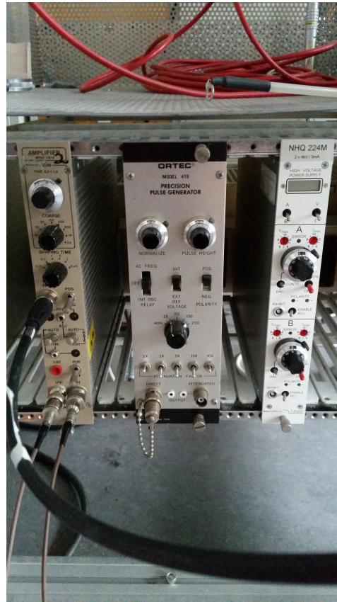
Figure 5.4: Picture of the components for readout and detector voltage supply mounted into a NIM Crate, from left to right, the Silena Milano Amplifier Model 7614, ORTEC model 419 50 Hz pulser and the high voltage supply NHQ 224M module.
