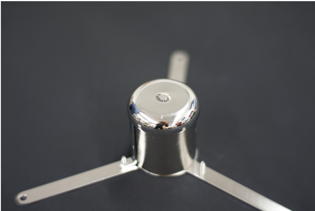
Figure 5.5: Close up of the magnet cap of the source, showing the annulus opening inside the cap, allowing for the electrons to pass through. The source material as well as the holding material are visible and show the off axis implementation of the source.
