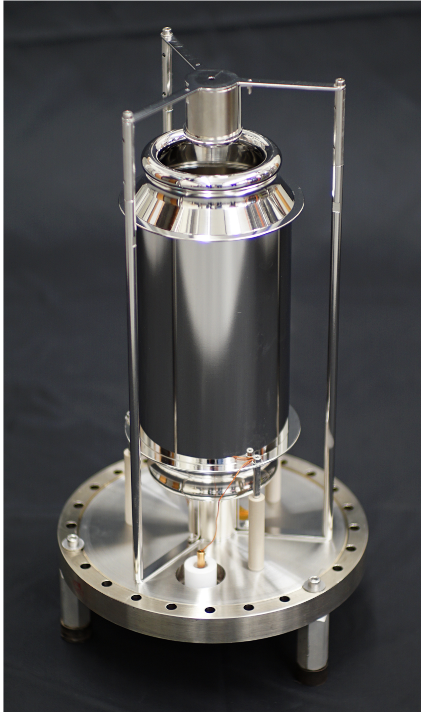
Figure 5.9: Picture of the electrode structure implemented in the laboratory in Münster. Visible are the central electrode, the poles that connect the magnet holdings and the magnets under the caps that fixate them.
