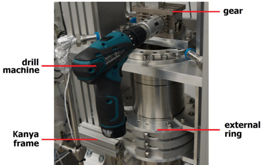
Figure 3.9.: Construction to couple-in or decouple the piston from the external magnetic ring: The external ring is fixed by Kanya frames, and the piston can be moved via a threaded rod and a gear by a drill machine.
