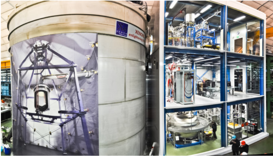
Figure 1.12.: The XENON1T Experiment underground. Left : the water tank with a poster showing the inside. Right : the three-story service building [XEN18].
