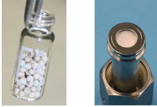
Figure 5.2: Left: ^{83}\text{Rb} source embedded in zeolite pellets. Right: Top of the rubidium source with the protective PTFE membrane filter[Han11].
