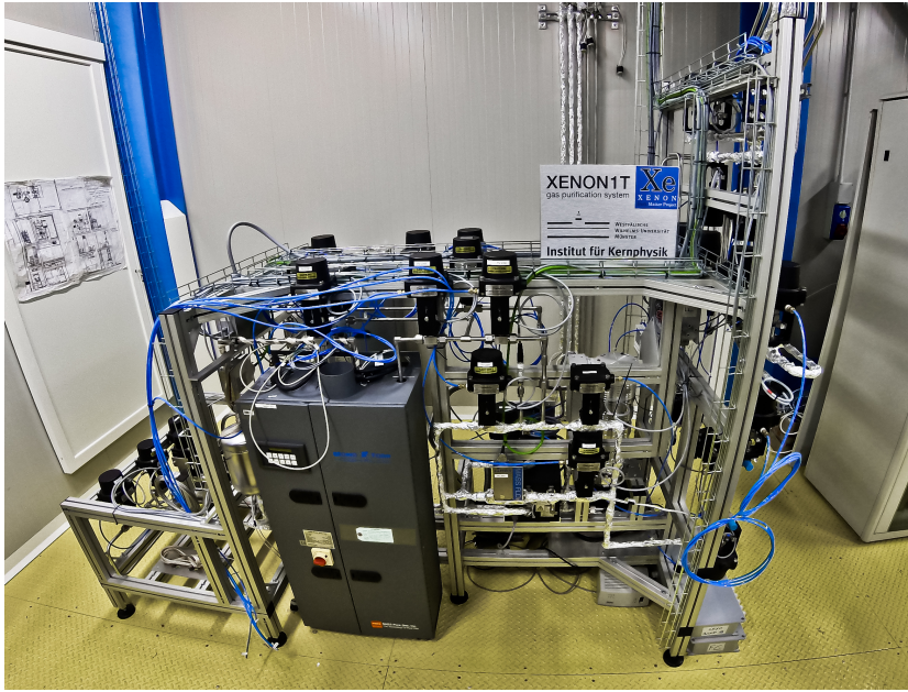
Figure 3.5: Picture of the purification system of XENON1T as installed at LNGS (courtesy of the XENON collaboration).
