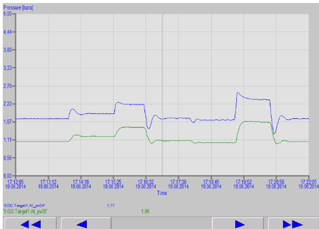
Figure 4.7: Time behaviour of inlet pressure (P204, blue) and outlet pressure (P205, green) while changing the inlet flow multiple times. The pressure difference of 700 mbar is accurately obtained within the order of seconds, even after rapid changes (compare t \approx 17:19:30 ).
