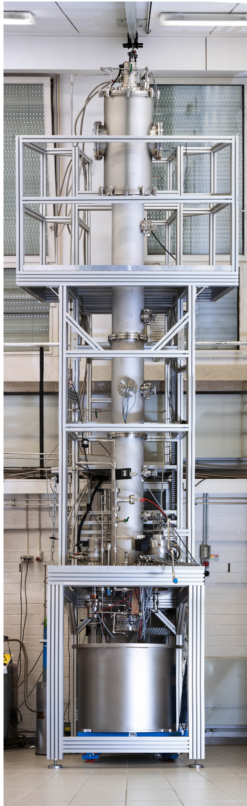
Figure 3.3: Picture of the 5 m distillation column developed for XENON1T in the university of Münster.
