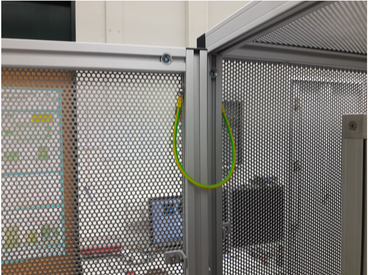
Figure 5.14.: The doors of the high voltage cage are grounded at two points with two independent cables, one at the top, the other at the bottom. The cables connect the KANYA profiles from the doors to the rest of the cage.
