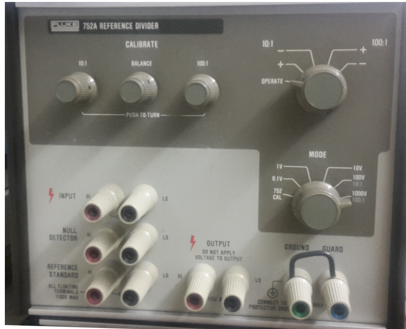
Figure 5.1.: Front panel of the Fluke 752A reference voltage divider.
