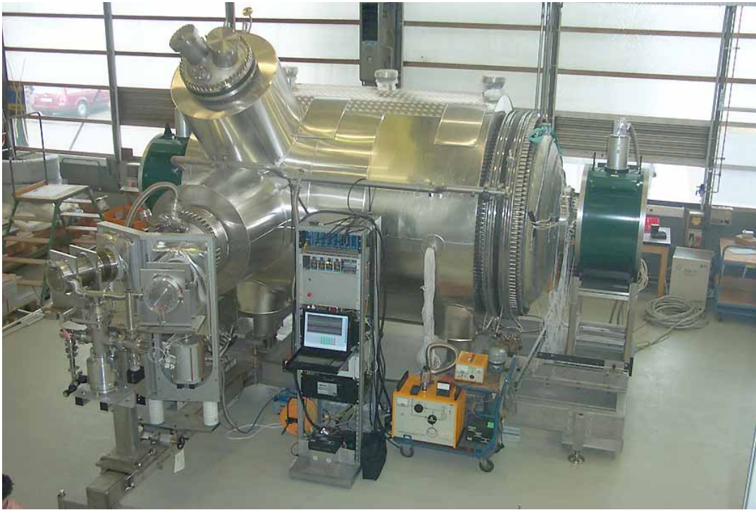
Figure 3.6.: The pre spectrometer of the KATRIN experiment consists of a cylindrical vessel (gray) with a simplified inner electrode system inside. At both ends of the vessel solenoid magnets are installed (green) to create a magnetic field, so that the spectrometer works as a MAC-E filter. [Kat04]
