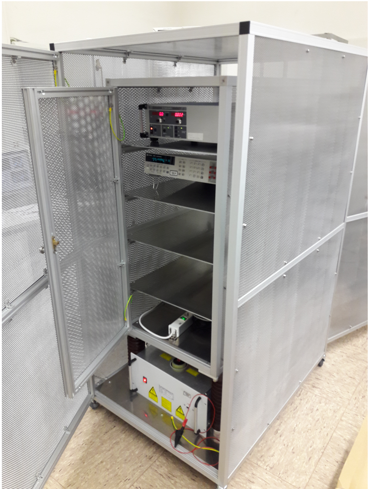
Figure 4.4.: This is the self made high voltage measurement cage. The inner cage has five shelves for the measurement equipment and stands on four insulators. Below the inner cage the isolating transformer is placed to supply the used devices inside the cage. The cage has a front and a back door to allow access to both sides of the cage. The cage was tested for high voltages of up to 35 kV.
