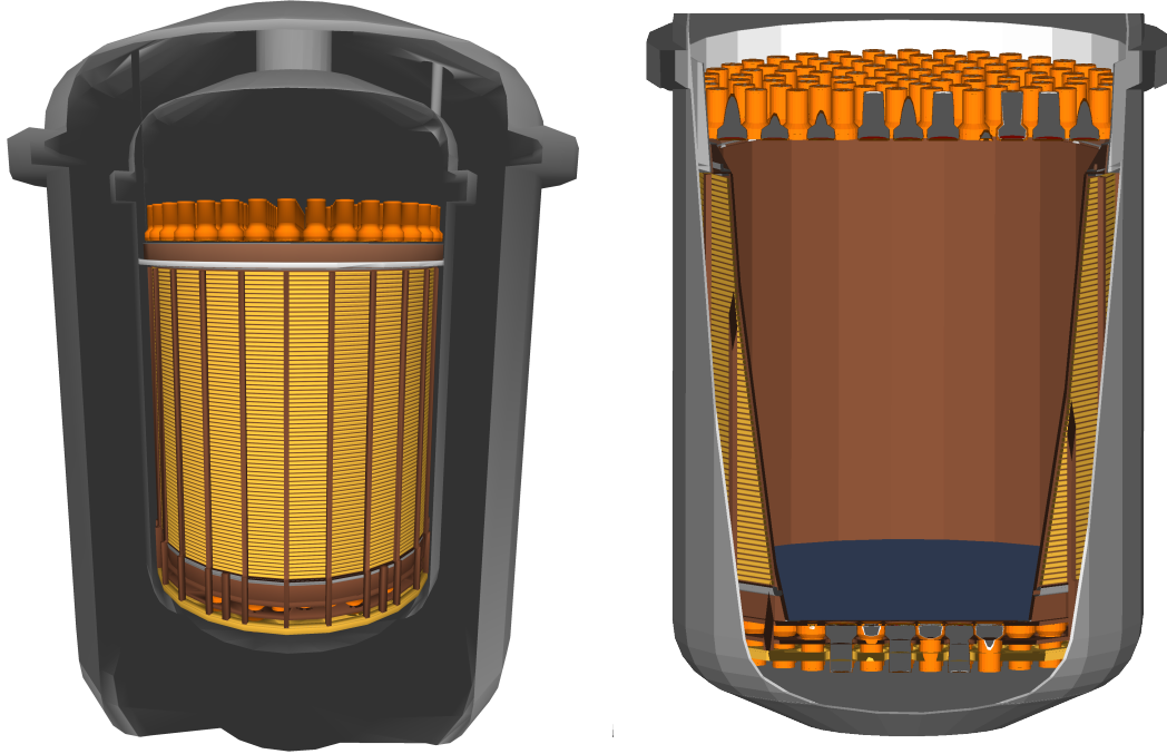
Figure 4.3: Direct view (left) on the XENON1T TPC with a top and bottom PMT array, a PTFE support structure (brown) and copper field shaping rings (yellow). The active LXe volume of the TPC is enclosed by a PTFE cylinder (right), the gate mesh (not visible, located right before the widening of the PTFE cylinder on top) and cathode (blue disk).
