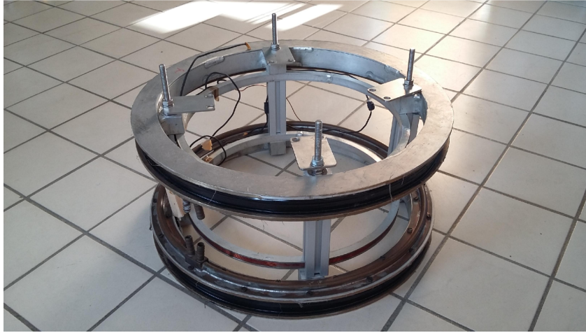
Figure 14: Picture of the solenoid coil system which was used in the lab experiments. The coils fit around the setup and can be attached to the mounting flange. It consists of two magnet pairs from which the outer and bigger coils were used in this thesis to create the magnetic field.
