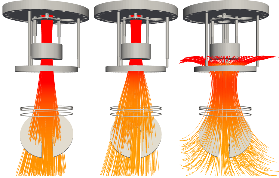
Figure 34: The picture shows three different configurations for the coil system. In the left one the field is created by a single coil covering only a small area of the cathode plate. The middle picture indicates the field for a two coil system where a small counter-rotating current is applied to the lower coil thus the field lines cover most of the cathode plate. The right picture shows the total compensation of the field by the lower coil, guiding the electrons away from the MCP.
