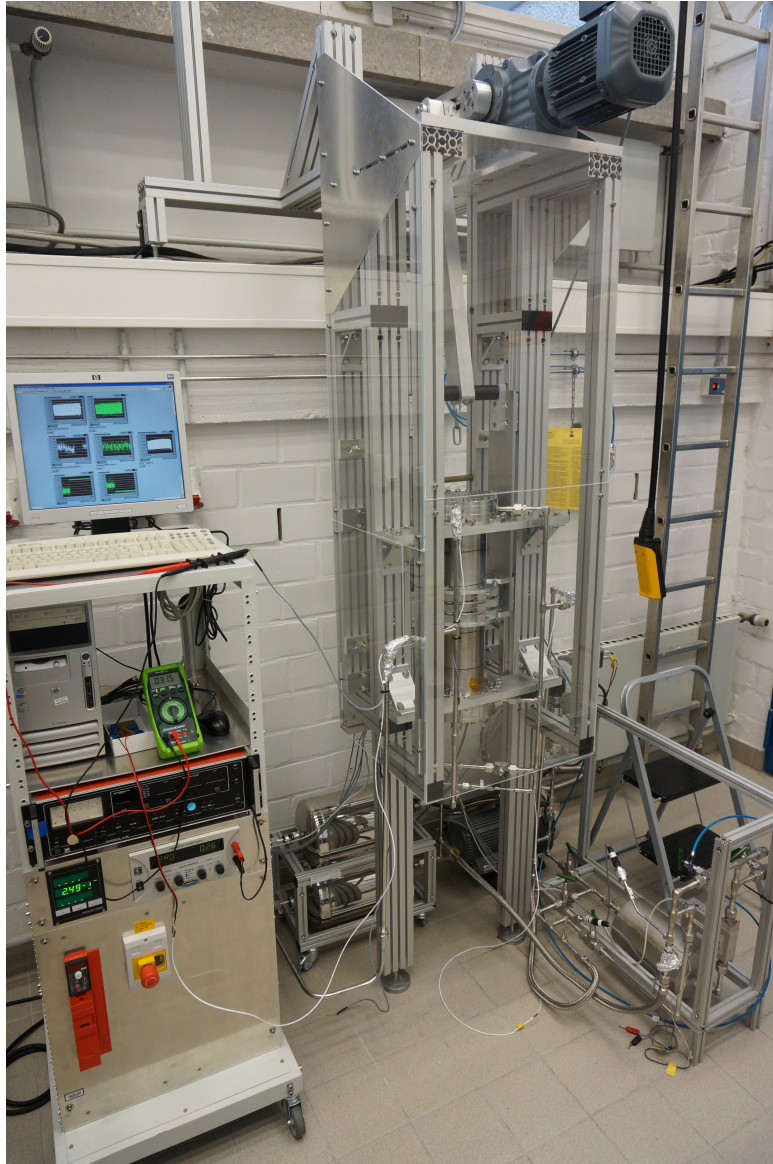
Figure 7.1.: Photo of pump setup. Left: control rack with PC for sensor read-out and a frequency converter to control the motor. Middle: the magnetically driven piston pump. Lower right: pump testing station. The gas system has a total volume of approximately 32l.
