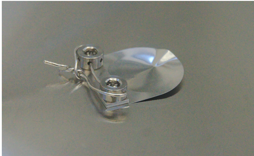
Figure 7.5.: Old flapper after less than an hour of operation. The plastic deformation leads to higher leakage.
