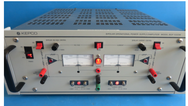
Figure 5.16: Front panel view of the Kepco Bop 1000m HV bipolar power supply appropriated to examine the transmission behaviour of the divider setup [Kep20].
