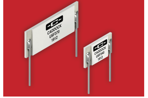
Figure 4.2: Model of the Caddock USF-300 Series ultra-stable low TCR ultra-precision metal film resistors. They are constructed with an aluminum oxide ceramic surrounding for high thermal conductivity [Cad20c].
