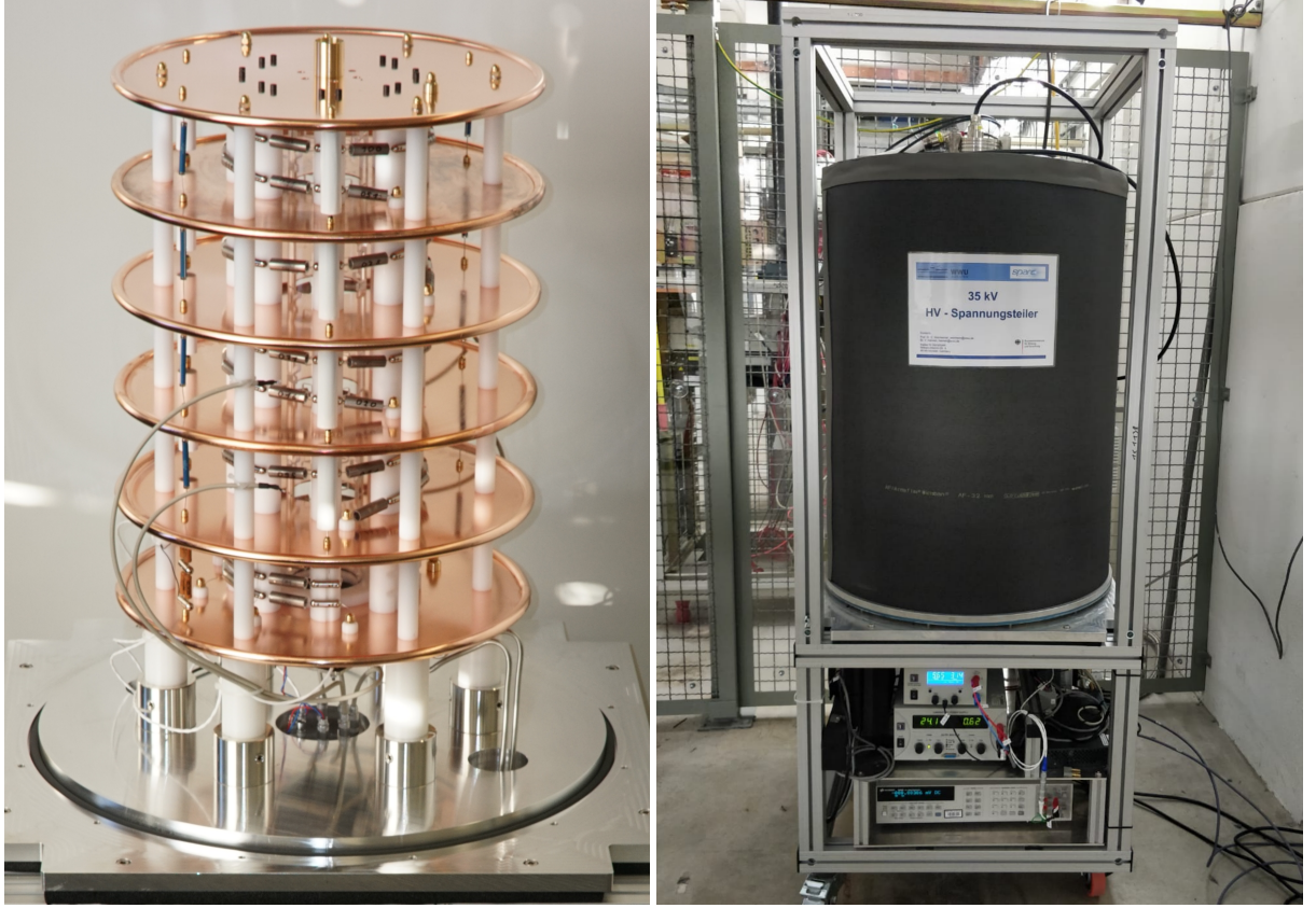
(a) Uncovered mechanical setup of the G35 HV divider staged on a stainless steel bottom plate. (b) G35 HV divider with stainless steel vessel and thermal insulation material coverage and periphery on movable KANYA profile.
