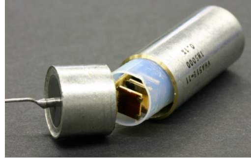
Figure 2.14: Inside view of a Vishay VHA518-11 resistor. It consists of several resistor chips made out of a ceramic substrate with a meander-type metal film on it. The chips are mounted inside a tinned brass cylinder filled with oil for better heat distribution [A + 15].
