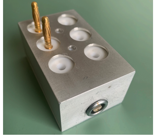
Figure 5.10: Custom banana plug to LEMO Series S adapter with shielding utilized for DMM measurements.
