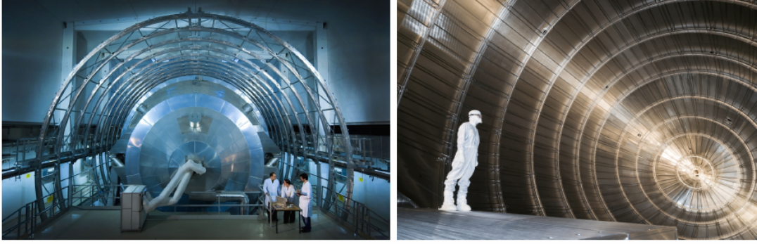
Figure 3.3: The main spectrometer. The left image shows the vessel viewed along the beam axis from the perspective of the detector end. It is surrounded by the air coil system. The right image shows the inside of the vessel, with the wire electrodes covering the inner surface. Figure from [KATb].
