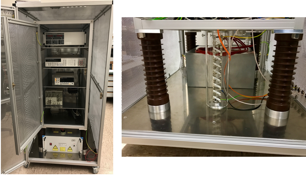
Figure 5.20: Picture of the custom-made HV cage. The inner cage can be operated on HV potential of up to 35 kV. The electrical devices within are supplied with power by an insulating transformer and controlled and read out via an optical link. In the right picture, the back-side of the cage can be seen, where the custom-made reference HV divider is installed.
