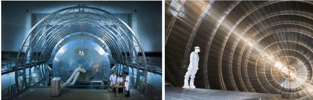
Figure 2.8: Main spectrometer. a) View from the detector to the source side along the beam axis. The air coil system surrounds the MS vessel. b) View from the inside showing the wire electrode system covering the whole inner surface. The images were taken from [34].
