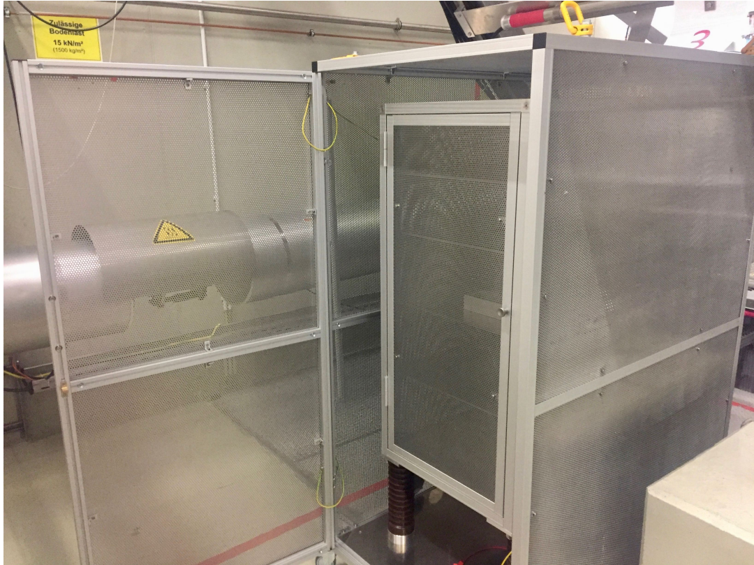
Figure 4.13: Picture of the HV cage installed at the basement of the main spectrometer. To the isolated inner cage a HV of up to -35\text{ kV} can be applied. The devices inside can be operated at this potential and are supplied with power by an isolating transformer, located at the basement. The outer cage is grounded and serves as protection against contact.
