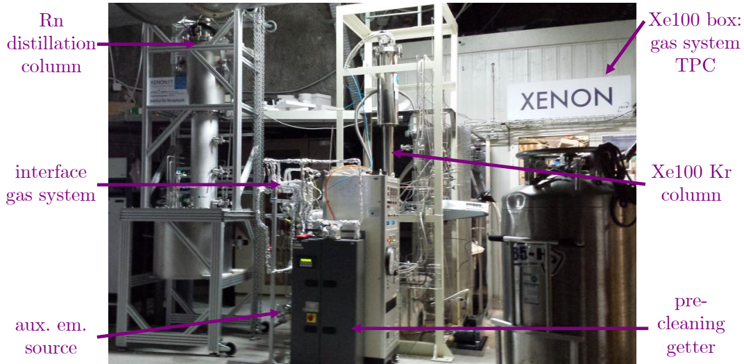
Figure 7.1: Experimental setup outside the XENON100 box: In the left, the modified distillation column for radon removal is installed next to the XENON100 krypton column. In the middle, the interface gas system with the artificial source is shown along with the getter for pre-cleaning of the new systems. On the right, the XENON100 box can be seen, housing the standard gas system and the detector system.
