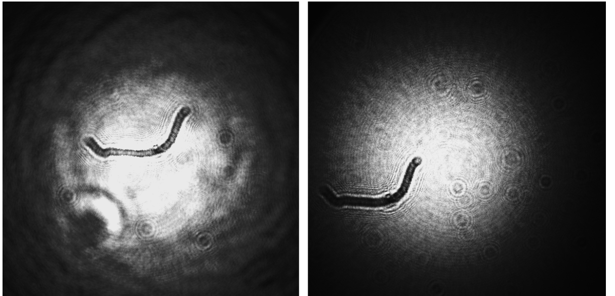
Figure 5.7 – Two laser beam profiles: On the left side with the old simple beam expander and on the right side with a spatial filter. Pictured in both images is an eyelash on the CCD camera. One sees a clearer beam profile on the right side even though some relics stay.
