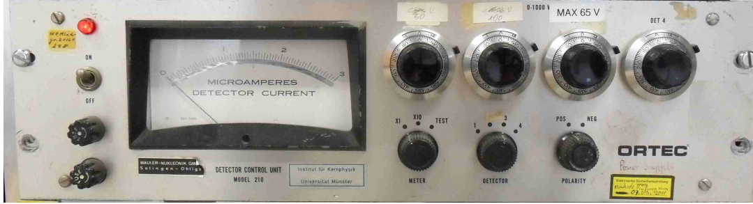
Figure 3.20.: Power supply ORTEC 210: The front panel dispose all control of the power supply. The Voltage range go from 0 – 1000 V disposed in four channels, the amplification factor is manual controlled with the Meter . The ammeter can be used in only in one channel, scaled in \mu\text{A} , also the power supply dispose the possibility to invert the current Polarity in positive or negative.
