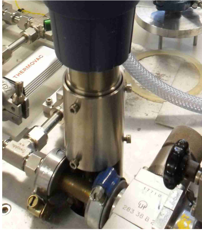
Figure 3.8.: Heat input for the spiral: Spiral of the radon trap is surrounding by a hollow cylinder, on the top of the cylinder a device to support a hot air gun has been developed. The hot air is injected on the central axis of the cylinder heating and reaching in around 10 min room temperature. Before the injection the gas will be sublimated using this configuration.
