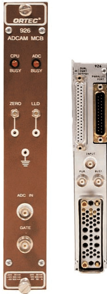
Figure 3.19.: Module ORTEC model 926 ADCAM multichannel Buffer : In this picture the front panel and the rear panel of the module Ortec 926 has been shown. In the front panel the manual controls of Zero and LLD can be observed, also the ground voltage is possible to adjust. In the rear panel the inputs Gate , PUR , and Busy can be found. The data outputs are the Parallel port , it is a standard IBM PC printer port and the Dual-port memory , it is an optional 37-pin connector provides the PC with a communication link and direct access to the Model 926's internal data memory. [Ortb]
