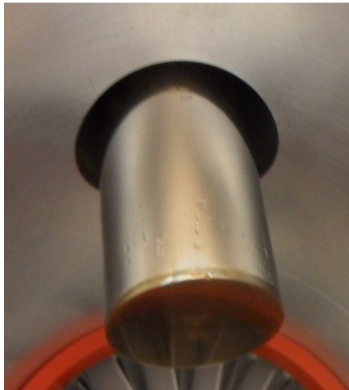
Figure 3.12.: Cold head: The cold head is a metal surface where a solid film of radon will be created. To cooling down this surface a cryogenic dewar flask is connected through a stem. The dewar flask is sealed and on top of the flask there is a gas output to decrease the pressure in the vessel. This setup is used to decreases the pressure in the dewar flask and to maintain a constant temperature in the cold head. The cold head is placed in the detection chamber and is used to create the solid sample injecting on the cold surface and to maintain the sample. Between the cold surface and the dewar flask a heater cartridge has been placed. This heater device disposes a PT100 thermometer included to monitor the temperature during the heating up. On the other side, the cold head disposes a PT100 to monitor the temperature on the metal surface.
