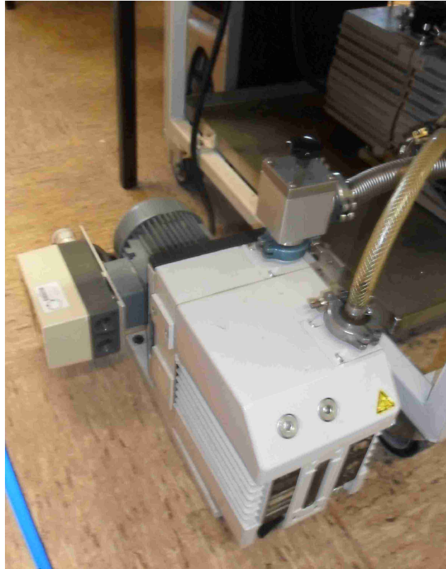
Figure 5.18.: Leybold pump. This pump was used to realize vacuum in the gas system after used the Alcatel pump. Leybold pump is a rotary pump with a pumping speed of 16.5 \text{ m}^3/\text{h} and an ultimate pressure of 2 \times 10^{-3} \text{ mbar} . This pump disposes a output without filter, so for this reason the output of this pump was redirect to the filter used by the other primary pump.
