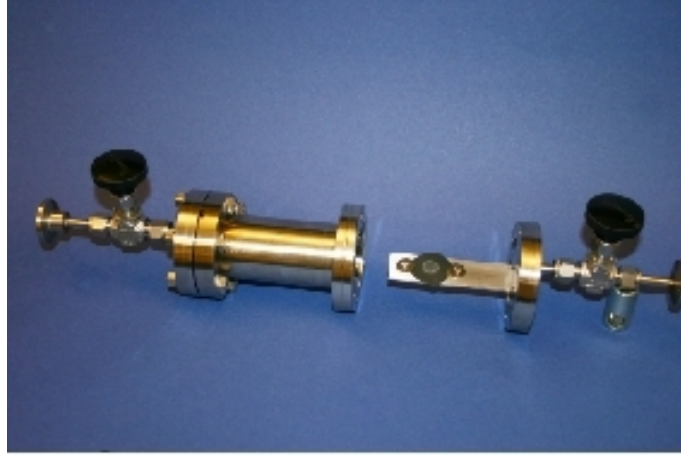
Figure 4.2.: Titan-Backing cylinder with the calibrated source ^{226}\text{Ra} . The radium source is the disc fixed in the central point. The radon gas will be contained into the cylinder. The cylinder disposes two valves to connect the air pump and plastic bag. Photo obtained by: [Nus11]
