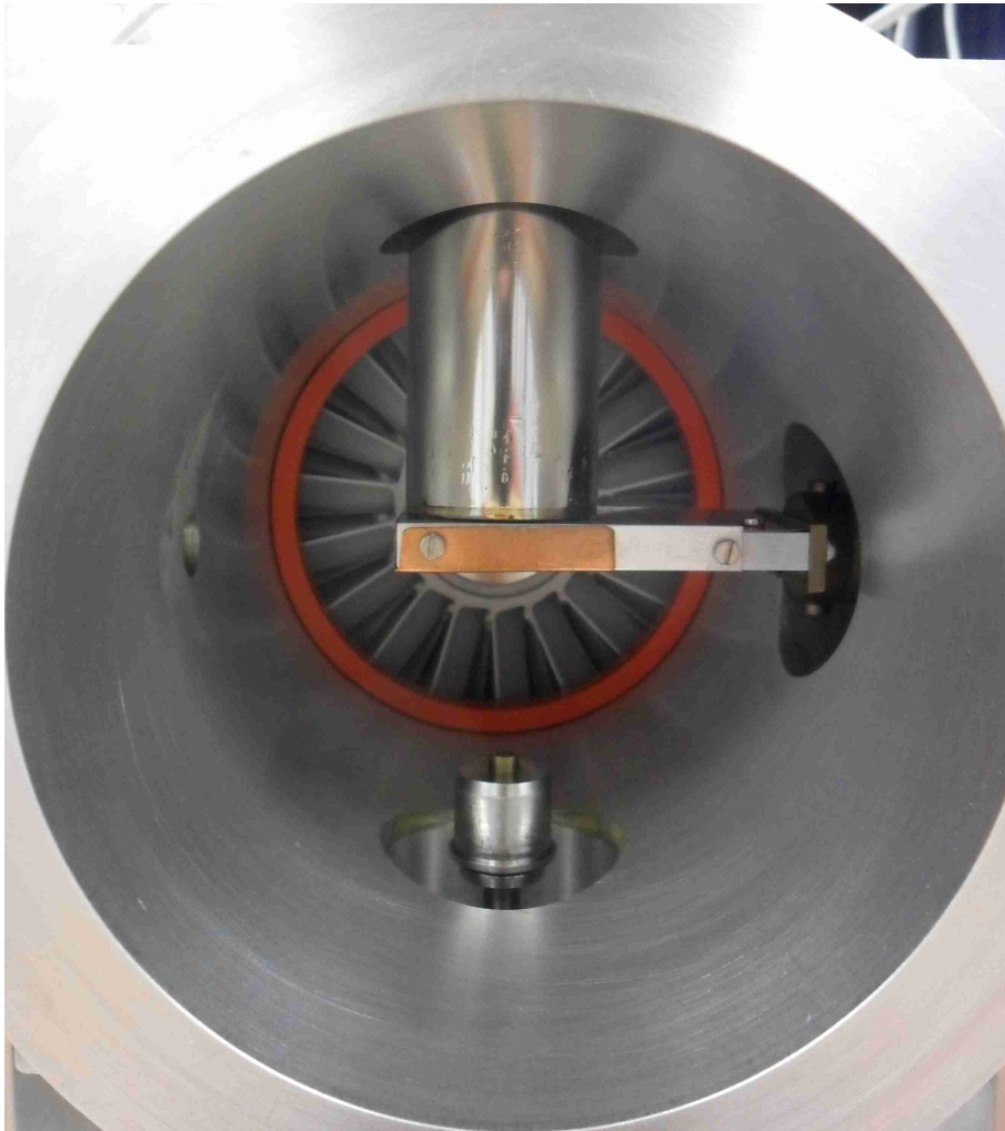
Figure 3.13.: Measurement configuration: In this photo the measure position can be observed. Created the radon sample on the cold head temperature must be maintained during the measurement at -204^{\circ}\text{C} . Finished the injection, the injector must be displaced to the position 0 mm. The injection process remains around 6 min, after the injection detector can be placed under the cold head to start the measurement.
