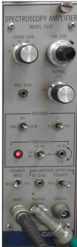
Figure 3.18.: Amplifier Canberra 2010: The amplifier is used to amplify and convert into a Gaussian pulse the original signal. The amplifier disposes an amplification from \times 10 to \times 3000 . The Pole zero can be adjust, as well as the Gaussian shaped using time constants of 0.25, 1, 2, 4, 8 or 12 \mu\text{s} . The input accepts positive or negative linear pulses with amplitude 0 V to \pm 12 V. Disposes an unipolar output with delayed 2 \mu\text{s} and \pm 10 V full scale linear output, and a bipolar output with a double differentiated linear output and +10 V full scale linear output.
