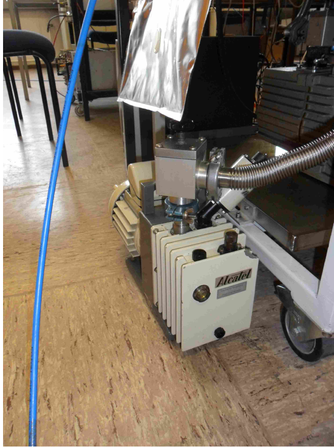
Figure 5.17.: Alcatel pump was the original pump of the gas system. The Alcatel pump is a rotary oil pump used to do vacuum in the gas system. A original point of this master thesis was checking the global efficiency of the system using this pump. But due to mechanical problems as well as blocking and lost of oil the pump was replaced for the Leybold pump.
