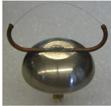
Figure 4.4. Wire initially used with semicircular shape and features: size 10\ \mu\text{m} and composition of tungsten (gold-plated).
