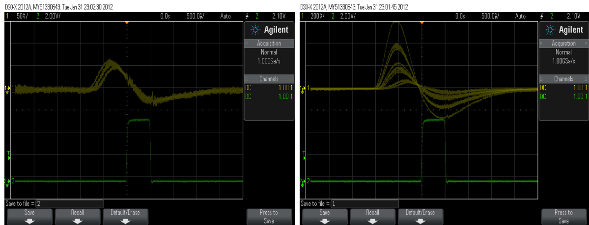
Figure 6.2. Signals expected at the output of both amplifier and discriminator respectively in the left-hand side of the picture. The amplifier gives output signals with nearly Gaussian shape, while the discriminator produces rectangular signals. In the right-hand side, amplifier output signals in CH 1 and discriminator's in CH 2 for the ^{241}\text{Am} source measured. Several amplitude values are observed.
