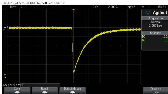
Figure 4.8. Preamplifier output signals. The signals can be visualized using an oscilloscope that allow to measure both amplitude (y-axis) and time (x-axis). The rise time of the output pulse is kept as short as possible ( \sim 10 - 100 ns), consistent with the charge collection time in the detector itself. The decay time of the pulse is made quite large (typically 50 or 100 \mu s) in order to get full collection of the charge from the detector, which produce pulses of \sim 0,01-1 \mu s.
