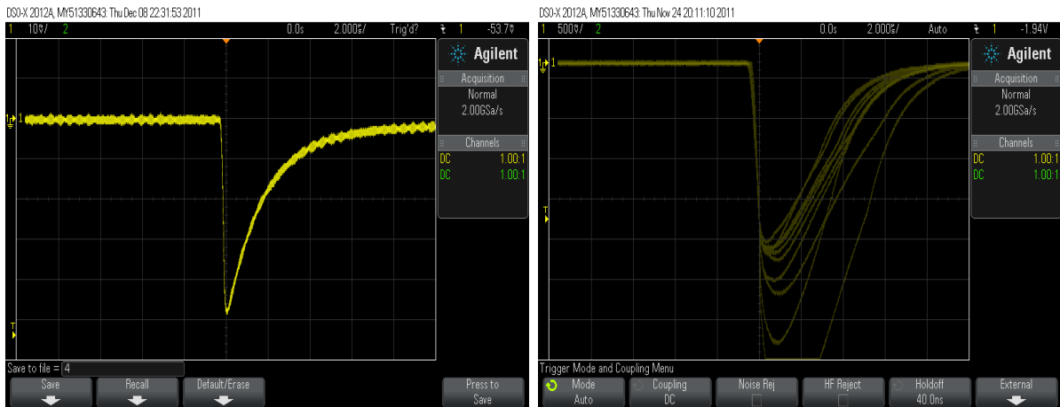
Figure 6.1. Output signals from the preamplifier expected for a monoenergetic source in the left-hand side of the figure and signals visualized for the ^{241}\text{Am} source on the oscilloscope with the available preamplifier on the right-hand side. Pulses of several amplitudes are observed for the monoenergetic \alpha source.
