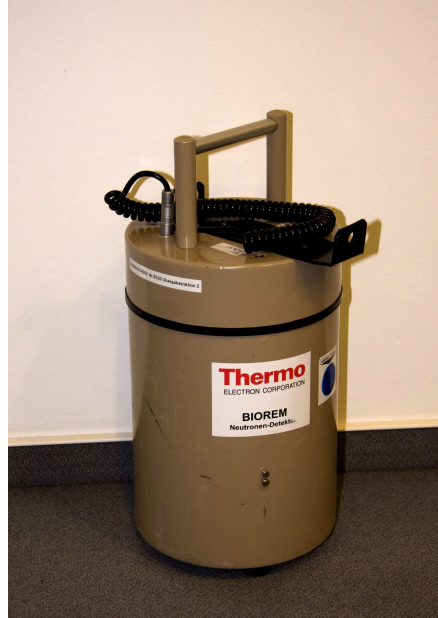
Figure 5.6: Figure of the intelligent neutron detector FHT (Biorem), which measures the neutron-ambient dose rate.
