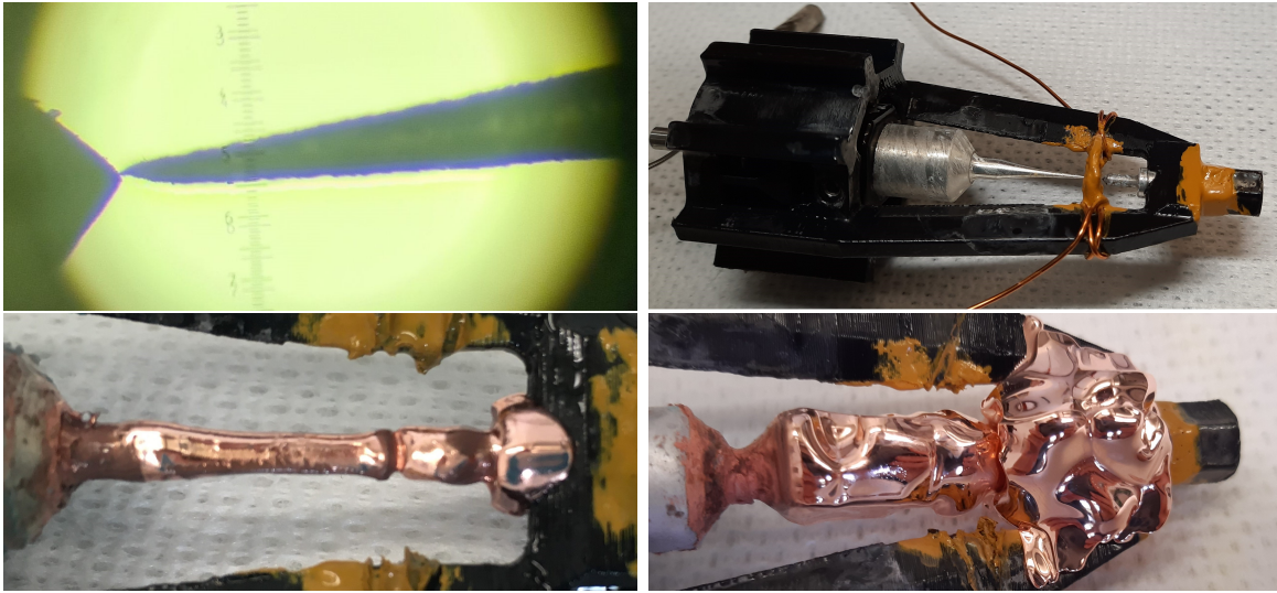
Figure 4.9: Example of a galvanization process, here for the cross section Q2103. Upper left: Adjustment of the two nozzle negatives under a microscope. The inlet negative (left) is fixed while the outlet negative (right) can be adjusted in distance and in both directions. Upper right: Placement of the auxiliary anode close to the narrowest diameter. As only ions from the inner face of the ring should detach, a yellow insulation lacquer covers the other faces. It is also used to attach the ring to the holder as there is no dedicated fixture. This piece is then galvanized. Lower left: Galvanized workpiece after a few days. The auxiliary anode is removed. Only a small notch close to the narrowest diameter of the nozzle forms which is already an improvement to previous galvanizations. The even and shiny surface shows that the bath properties were kept in the right range. Lower right: Final galvanization workpiece. The outer geometry is now manufactured by the mechanical workshop.
