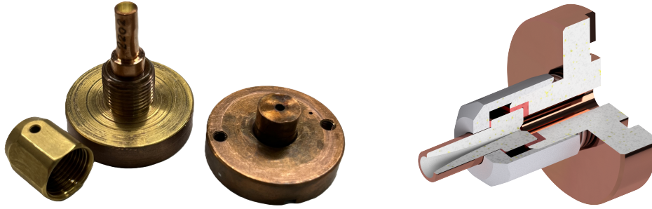
Figure 4.16: The two different outer nozzle geometries and the adaption with a nozzle adapter are depicted. Left: Small nozzle 2202 in nozzle adapter with the tightening nut aside and large A19 nozzle. The A19 nozzle was shortened in [Ves18], so that it only has a total length of 14 mm. Right: CAD drawing of a small nozzle in the nozzle adapter. Nozzle adapter and large nozzle can be placed in the nozzle holder within MCTs. The sealing for all nozzles used in this thesis and the nozzle adapter is made of polyimide. For other nozzles, e.g., the CERN nozzle a sealing with indium is foreseen. The small nozzle is sealed in the nozzle adapter with a further polyimide layer and tightened with a nut.
