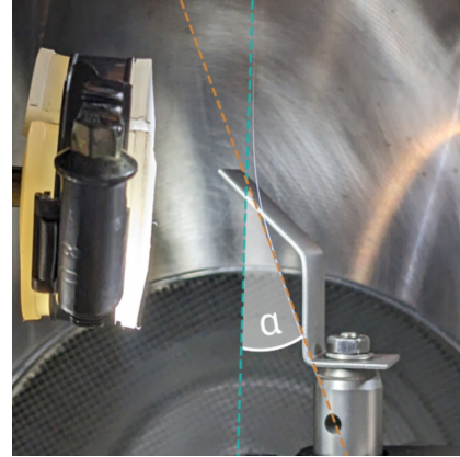
Figure 4.41.: Determination of bending angles through aligning tangents to the beam. [Hann 24]
