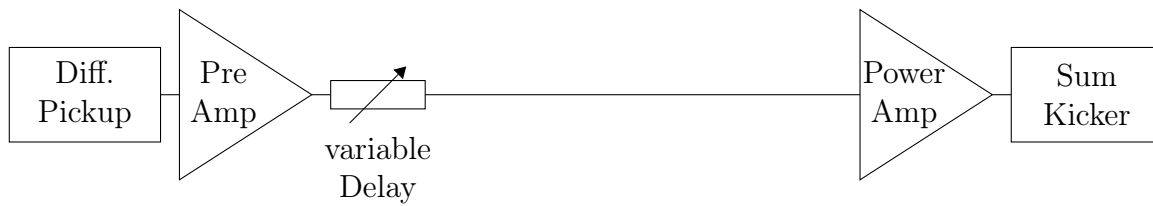
Figure 4.7: Schematic drawing of the electronic setup for the Palmer method. The differential signal from the pickup will be used, as it contains the information of the transversal deviation, which is proportional to the longitudinal deviation when the pickup is placed in a section with high dispersion. This signal is pre-amplified and delayed to match the phase at the kicker. Afterwards, it is amplified and fed as sum signal into the kicker, so that the momentum is corrected here (based on [SKM16]).
