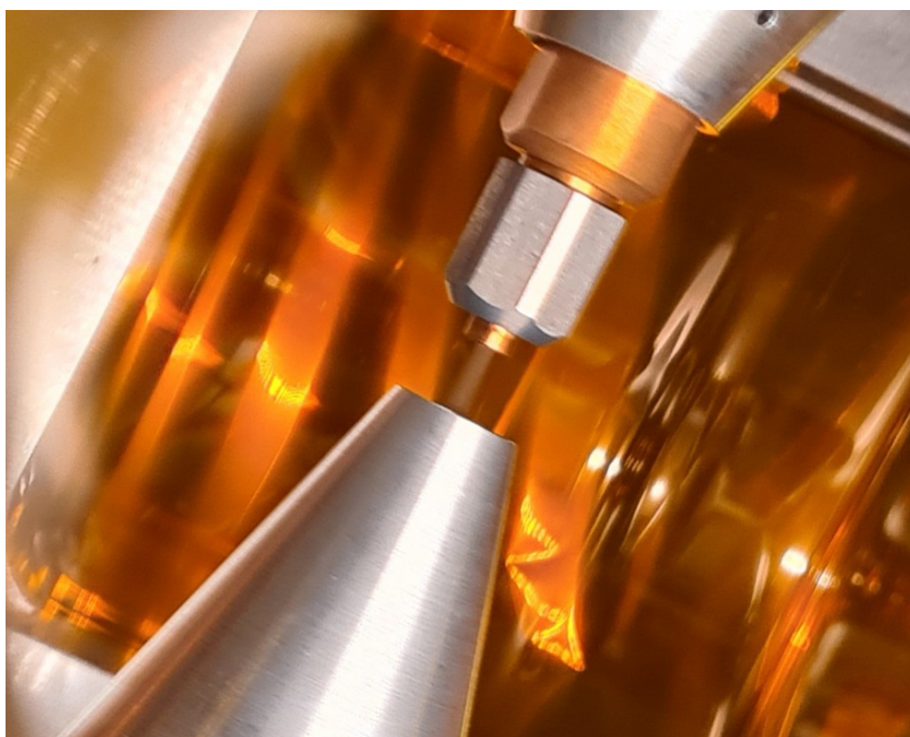
Figure 7.19: Photograph of the argon jet leaving the nozzle of the jet target from top to bottom. Below the nozzle it enters the catcher and is pumped away by the pumping station. The picture was taken through a small vacuum window. In the background, the Mylar window of the chamber towards spectrometer B of the A1 experiment can be seen.
