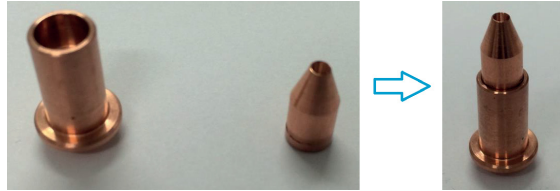
Figure 3.6: The final Laval nozzle for the jet target MCT-M for the MAGIX experiment. Left: The nozzle holder (right) and the Laval nozzle (left) which is shrunk on the nozzle holder. Right: The final nozzle consisting of the Laval nozzle and the nozzle holder. Pictures taken by D. Bonaventura.
