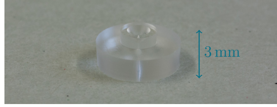
Figure 3.3: Picture of the glass nozzle manufactured by the selective laser-induced etching of glass. The size of the nozzle is limited by the used optics. Picture taken by D. Bonaventura.
