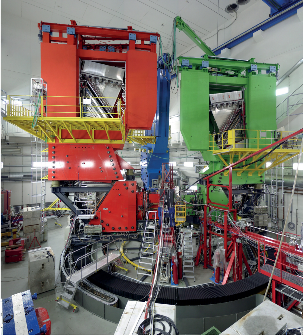
Figure 6.13: Photography of the A1 hall with the three spectrometers A (red), B (blue), and C (green). The electron beam direction is from bottom right (red frame) to the gap between spectrometer A and B. The scattering chamber with the jet target will be installed in the center of the three spectrometers. Taken from [Wei03].
