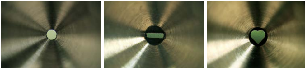
Figure 5.51.: Installed collimators with circular (diameter 0.5 mm), rectangular ((780 × 190) μm 2 ), and heart shaped opening (maximal length 760 μm 2 ).
