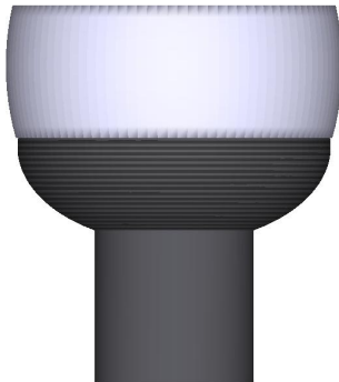
(a) Ellipsoidal reflector with a = 70 mm and b = 55 mm.
