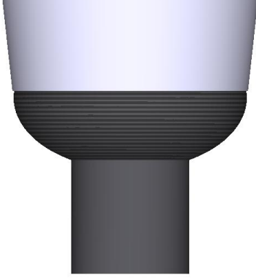
(a) Conical reflector with \beta = 10 degrees.
