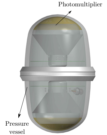
Figure 3.4. Dual optical sensor in an Ellipsoid Glass for Gen2 (D-Egg). A digital optical module designed for IceCube Upgrade. Courtesy of the IceCube Collaboration.
