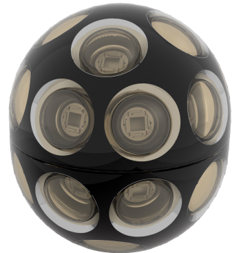
Figure 3.12: Representation of the multi-PMT Digital Optical Module (mDOM). Courtesy of IceCube collaboration [44].
