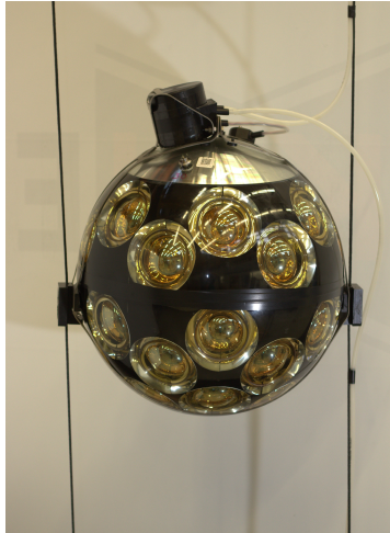
Figure 9: Km3NeT multi-PMT digital optical module containing 31 3-inch PMTs in a spherical pressure vessel. Taken from [26].
