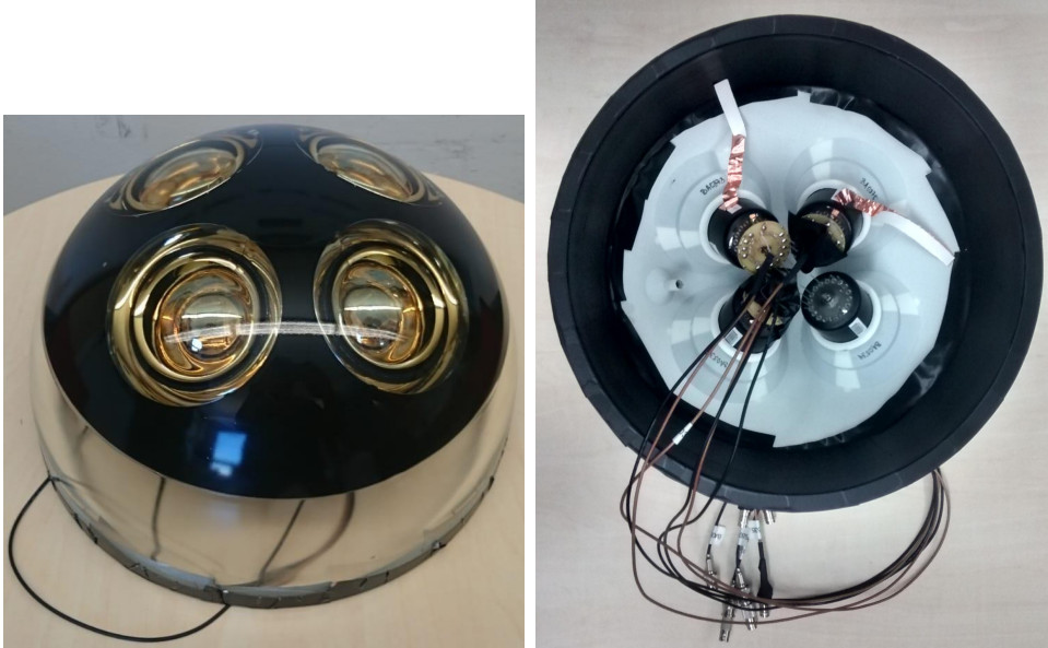
Figure 49: Experimental setup with four PMTs with reflectors and holding structure in a glass vessel to test the calibration method. Between the glass and the other components is a layer of gel. Left: without black tape from the front. Right: glass vessel in black tape from the back.
