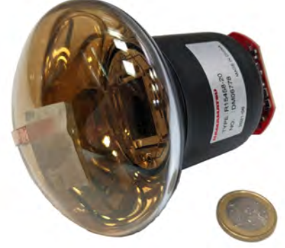
FIGURE 3.6: Hamamatsu R15458-20 PMT with integrated active base used in the mDOM. Figure taken from [36].
