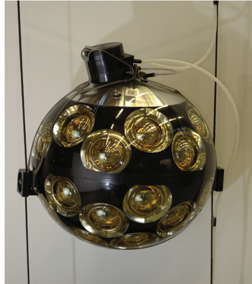
Figure 2.13: KM3NeT multi-PMT digital optical module mounted between two dyneema ropes and connected to an electro-optical cable via a break-out box. Shown is the final configuration before deployment. Photo taken from [104].
