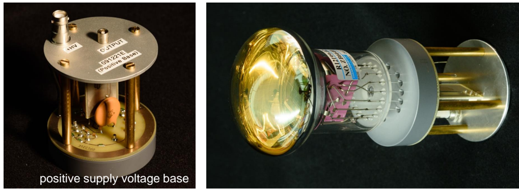
Figure 6.4: Resistive positive supply voltage base. The device was produced based on the circuitry presented in figure 6.3. Note the characteristic large capacitor used for the decoupling of the output.
