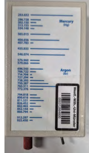
FIGURE 4.2.1: Photograph of the calibration lamp.
