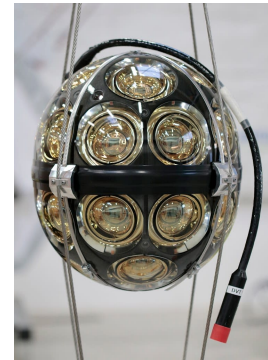
FIGURE 2.5.2: mDOM with harness consisting of 24 PMTs. Taken from [31].
