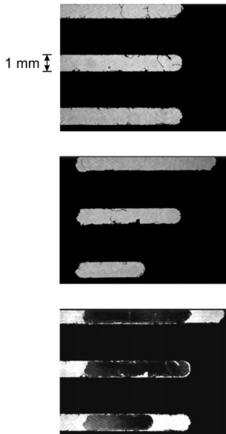
Fig. 12. Experimental result of object comparison. Top : master object. Middle : object under test. Bottom : detected output
