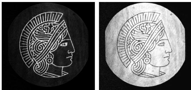
Fig. 10. Example of inversion of an analog data page realized by subtraction of the data page from a plane wave stored in the volume holographic memory.
